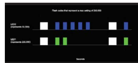
Figure 1 To change the maximum gallons setting, press and hold the button for 1 second. LED1 should turn solid green, LED2 should turn off and LED3 should flash green the number of times that corresponds to the current setting. Pressing the button for less than 1 second would increment the value, rolling over from 9 to 0. Below, Figure 2, is an example of the LEDs in this mode.
