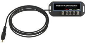
**REMOTE ALARM CONNECTION MODULE:** Allows for a connection to a remote device such as a buzzer, light, alarm system, PLC, etc., via a pair of contacts. In normal operation the OK and COM contacts will be connected, and in a fault condition (Low UV, Lamp fail, Power Fail), the Fault and COM contacts will be connected. Maximum contact rating is 30V / 1A (use 16-22 AWG). Order PN **SPRW-MOD-RAM**.
