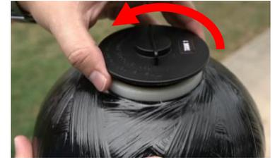
1) Unscrew the cap on top of the carbon filter tank.
