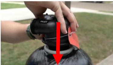
5) Press the tank head down to allow the threads to catch.
