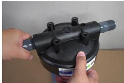
28) Install a PVC nipple onto each the inlet and outlet of the sediment filter housing. Fully tighten using pliers avoiding damage to the threads on the PVC nipples.
