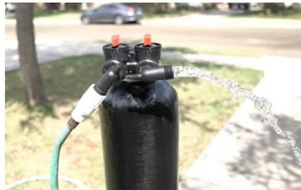
20) Flush with water in the opposite direction until the water runs clear. Approx. 3-5 min. Once done the hose and hose bib assembly can be removed.
