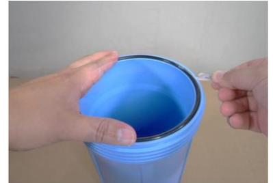
23) Squeeze lubricant onto the O-ring then spread it using your finger.
