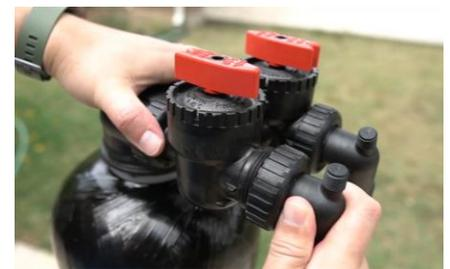
12) Attach and tighten a MNPT Fitting onto the connections on each of the bypass valves.
