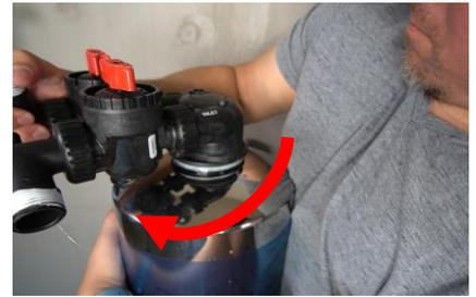
Fully re-tighten the head onto the tank. The O-ring will now be able to reset.
