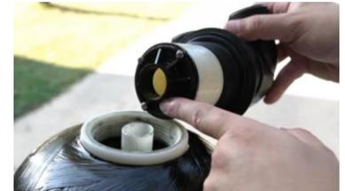
4) Align the opening on the bottom of the tank head with the pipe inside the tank.
