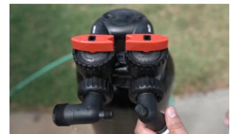
15) Switch the tank to bypass and store for 48 hours.
