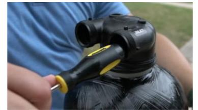
7) Insert a blunt tool into one of the connections on the head. A screwdriver handle will work.
