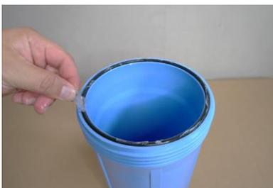
24) Flip the O-Ring over and lubricate the opposite side as well.
