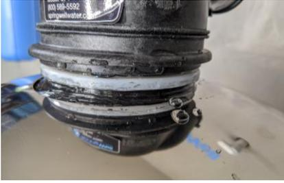
Water leaking from the tank head collar indicates the head is either not tight enough, or that the O-ring became bunched.
