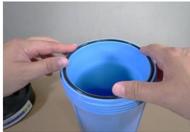
22) The O-ring will now be laid into the groove around the top of the sediment filter Housing tank.
